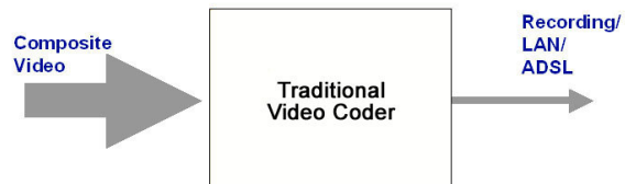
Fig.1 Traditional video coders - the single video stream is used for both recording and remote surveillance.
