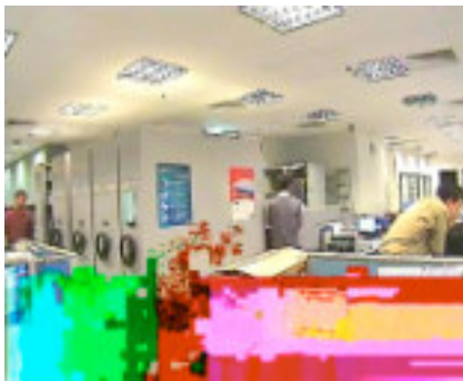
Fig. 5 Effects of transmission delay and/or error of a MPEG-4 coder in a busy Internet channel
